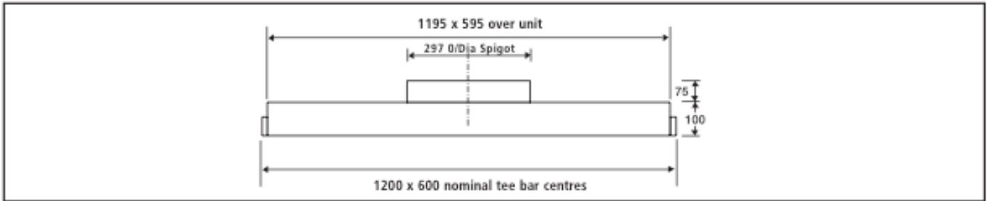
Section through model PAR single panel
